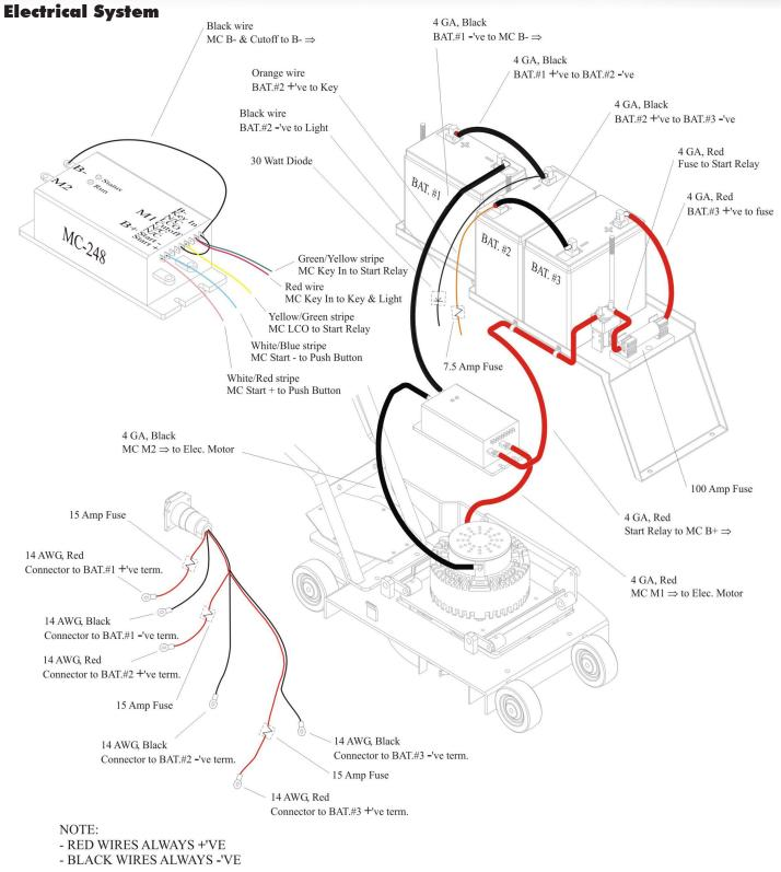
WARNING : INSTALLING BACKWARDS WILL CAUSE DAMAGE AND POSSIBLE INJURY.
