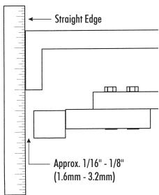
7. On the eight blade plate, we recommend every second blade be inset by moving it to the back of the slide groove. The alternate blade tips are positioned correctly by measuring from the outer edge of the blade guard casing to the tip of the blade. It should be 1/16" to 1/8" inside the edge.
